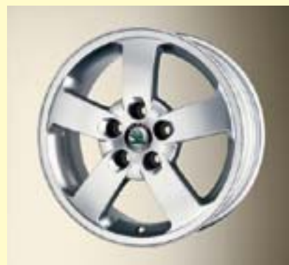
Alloy wheel 6.0J x 15" for tyre 195/50 R15 or 185/55 R15 (CCR 400 001)
