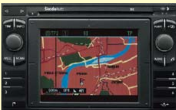
The navigation system includes TMC dynamic module and a radio (AAN 000 001)
